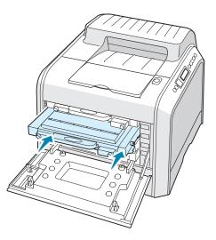
When the toner cartridges are correctly installed, the yellow and black cartridges are not fully inserted. These will be pushed into place when you close the left cover.
